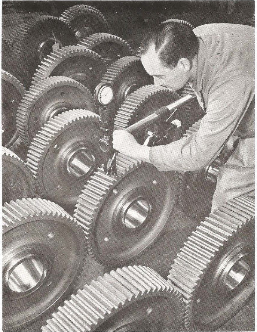
Measuring the hardness of a gear tooth flank with a portable tester. The apparatus clamps over a suitable number of teeth and gives a direct Rockwell hardness reading at various positions on the working surfaces.
